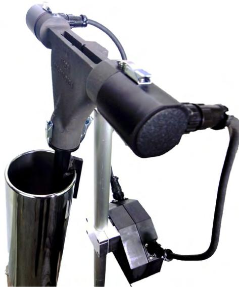
*Caution: Ensure the sensor head has been powered on and self-calibrated before affixing the sensor head to the exhaust. If you self-calibrate the unit while the sensor head is in the flow of exhaust, the equipment will see the exhaust, think the exhaust is the normal dust in the air, and call it zero.*
